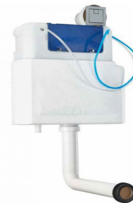
Premium Concealed Cistern Dual flush, Bottom inlet, Top & front access. Polystyrene jacket reduces flush noise. Modern square dual flush button
